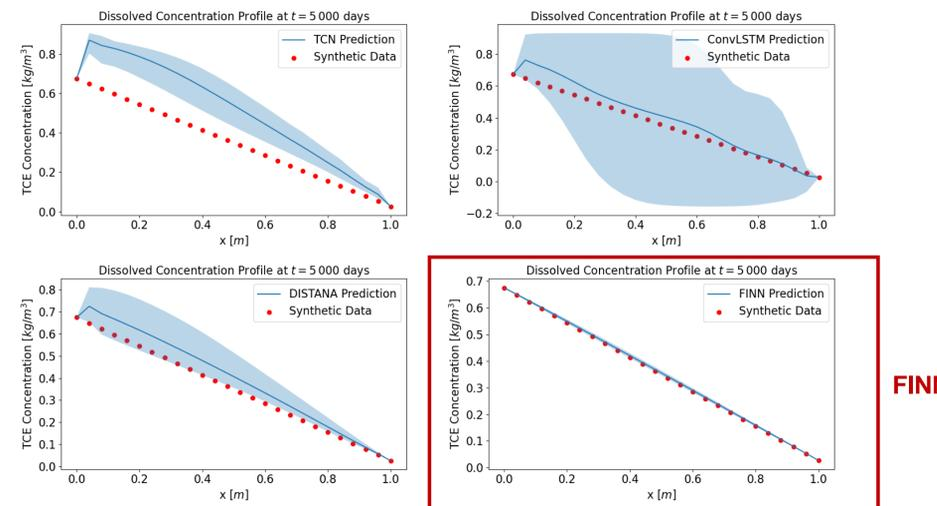
Dissolved concentration profile prediction mean (with confidence interval) at  $t = 5000$  days compared with the test dataset obtained using TCN (top left), ConvLSTM (top right), DISTANA (bottom left), and FINN (bottom right).
