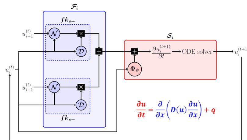
Illustration of the Flux and State Kernels in the FINN.
